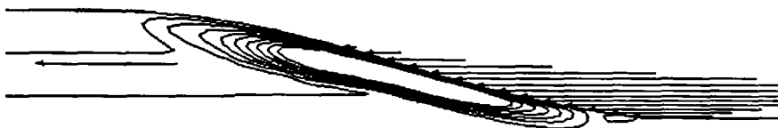
Figure 17 Streamlines with horizontal powder injection and \gamma_{lg} = 7 N/m
